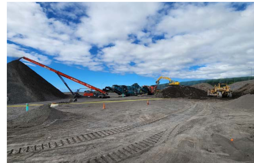
Stacker conveyor recently acquired by Nan, Inc. to increase Big Island crusher operation
