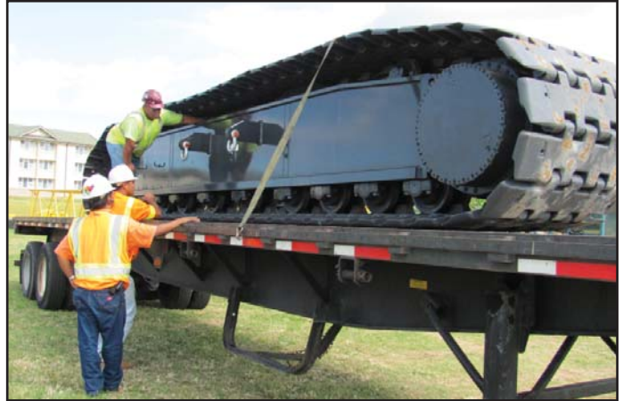
Workers inspect a new track for the CK2000.
